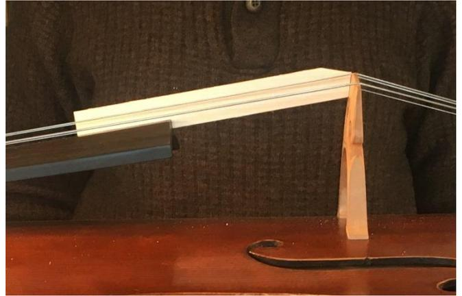
which is designed to fit precisely between the top of the bridge and the end of your fingerboard when the bridge is standing perfectly upright. Use this gauge to check the posture of your bridge and correct the bridge angle as required. Make sure the grooves are well lubricated with dry soap before you correct the bridge angle, otherwise the strings will grip the bridge too firmly to allow any movement.
